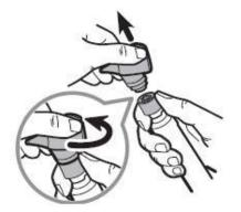
STEP TWO: Bulb located in the bottom portion of otoscope head (see arrow)
