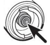
STEP THREE: Pull bulb out in direction of arrow below by pinching exposed portion of bulb with thumb and index finger (use or tweezers or similar tool)
